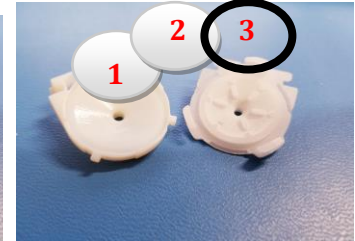
Step 3.9: Place sampling filter (1) (if performing gravimetric analysis), followed by a clean protection filter (2), followed by the O-ring (3) in the smooth cavity of the filter cartridge. The filters and O-ring must be placed in this order in the smooth cavity.
