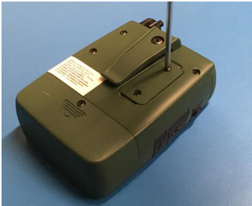
Step 3.1: Loosen filter cartridge cover screws with a small Philips screwdriver
