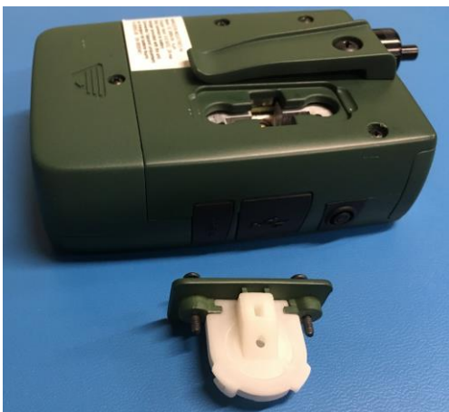
Step 3.4: Filter cartridge and cover fully extracted from the DustCount
