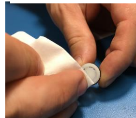
Step 2.2. Use a fiber-free cloth (Kimwipes) soaked in alcohol to remove any visible dust on the white porous surface.
