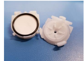
Step 3.7: Separate filter cartridge halves exposing O-ring and filter(s)
