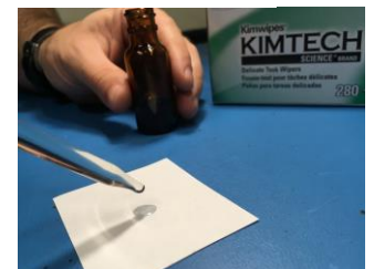
Step 2.3 Use the Impactor Oil Applicator to apply one drop of oil to a fiber-free paper pad.
