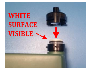
Step 2.5 Place impactor plate back in the holder ensuring white surface is oiled and aligned away from the DustCount.
