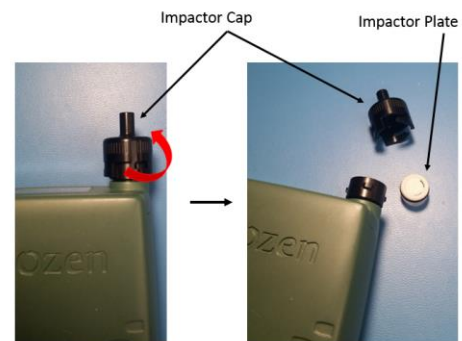
Step 2.1 Twist off Impactor cap and remove impactor plate assembly from the holder.
