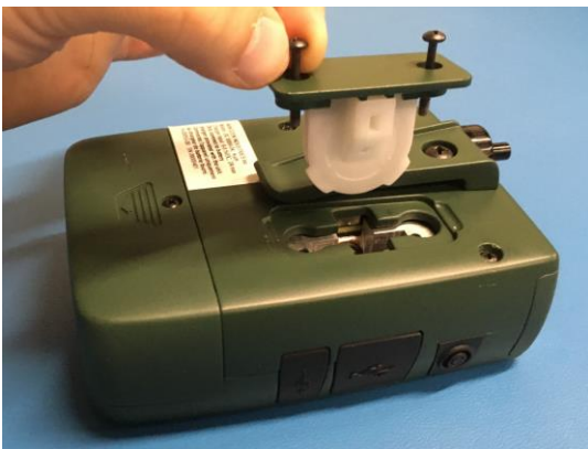
Figure 8. Extract filter Cassette by pulling up on the screws
