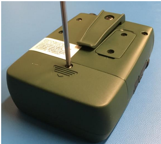
Figure 44. Loosening and removing Screw for Rear Battery Cover
