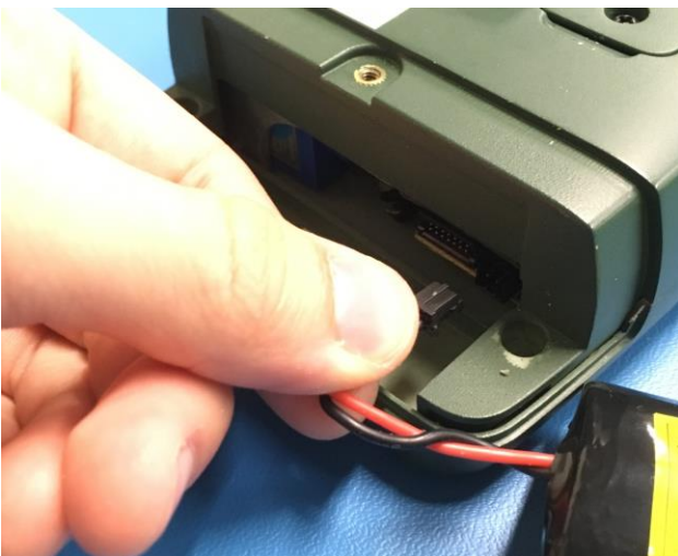
Figure 47. Disconnecting or re-connecting Battery
