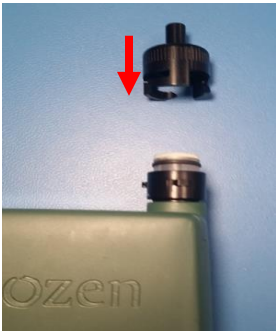
Figure 6. Place Impact Plate Back into the Holder.
