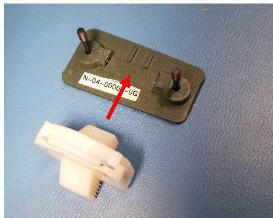
Figure 14. Press the Cassette Halves Together in Several Places, then Slide the Cassette onto the Cover.
