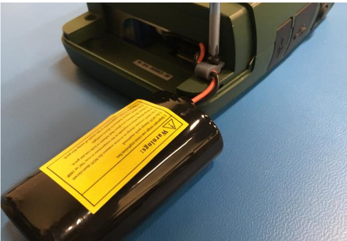
Figure 46. Removing Screw to release Battery Cable Tie
