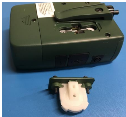
Figure 7. Loosen filter Cassette cover screws with a small Philips screwdriver
