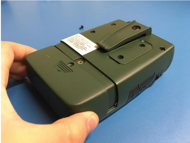
Figure 45. Sliding Off Rear battery cover
