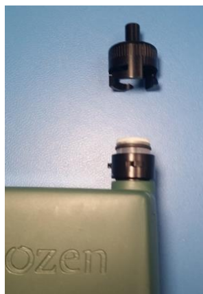
Figure 5 Re-installing impactor plate
