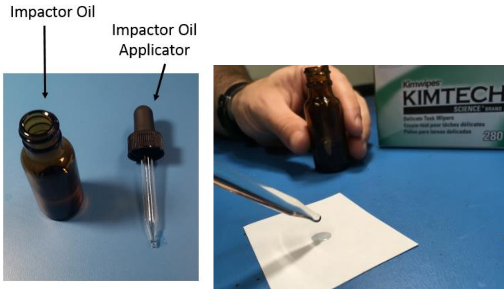
Figure 3 Applying oil to fiber-free pad
